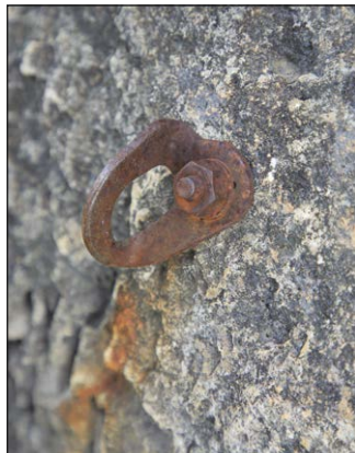
A rusty bolt - probably sound but difficult to trust
